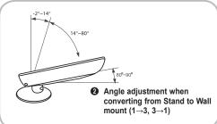
Figure ② shows the adjustment angle (14°~80°)
